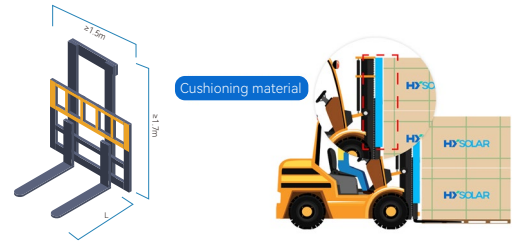
Forklift truck mast: height \geq 1.7M , width \geq 1.5M ; cushion materials such as EPE or rubber cushion shall be placed in front of the forklift truck mast
